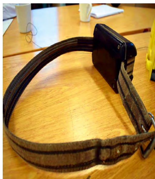
Cow collar with the sensing unit
