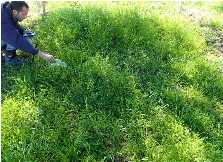
Figure 5. Measuring Photosynthetically Active Radiation (PAR) and leaf area index (LAI) with a Sunscan light meter within the shaded plot
