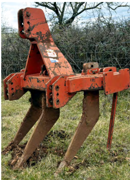
This decompactor with 3 teeth is fissuring the ground to a depth of 40 cm
