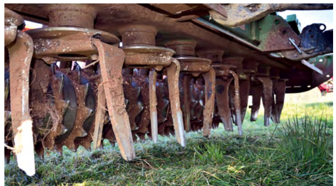
The rotary tine harrow levels the ground effectively and makes the particles thinner
